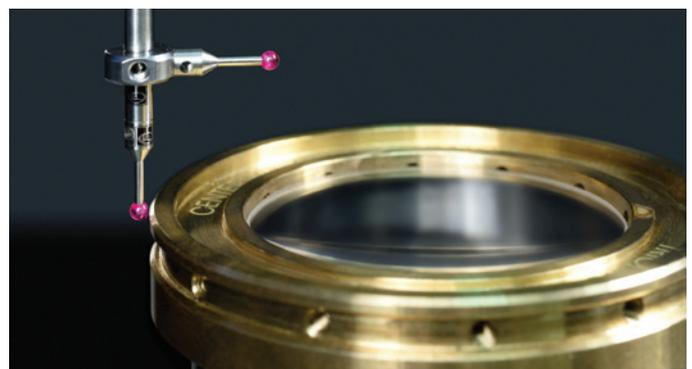
*Unequaled repeatability and scalability result from integrated metrology in the ATS 200 alignment turning machine (photo courtesy of TRIOPTICS GmbH)*
