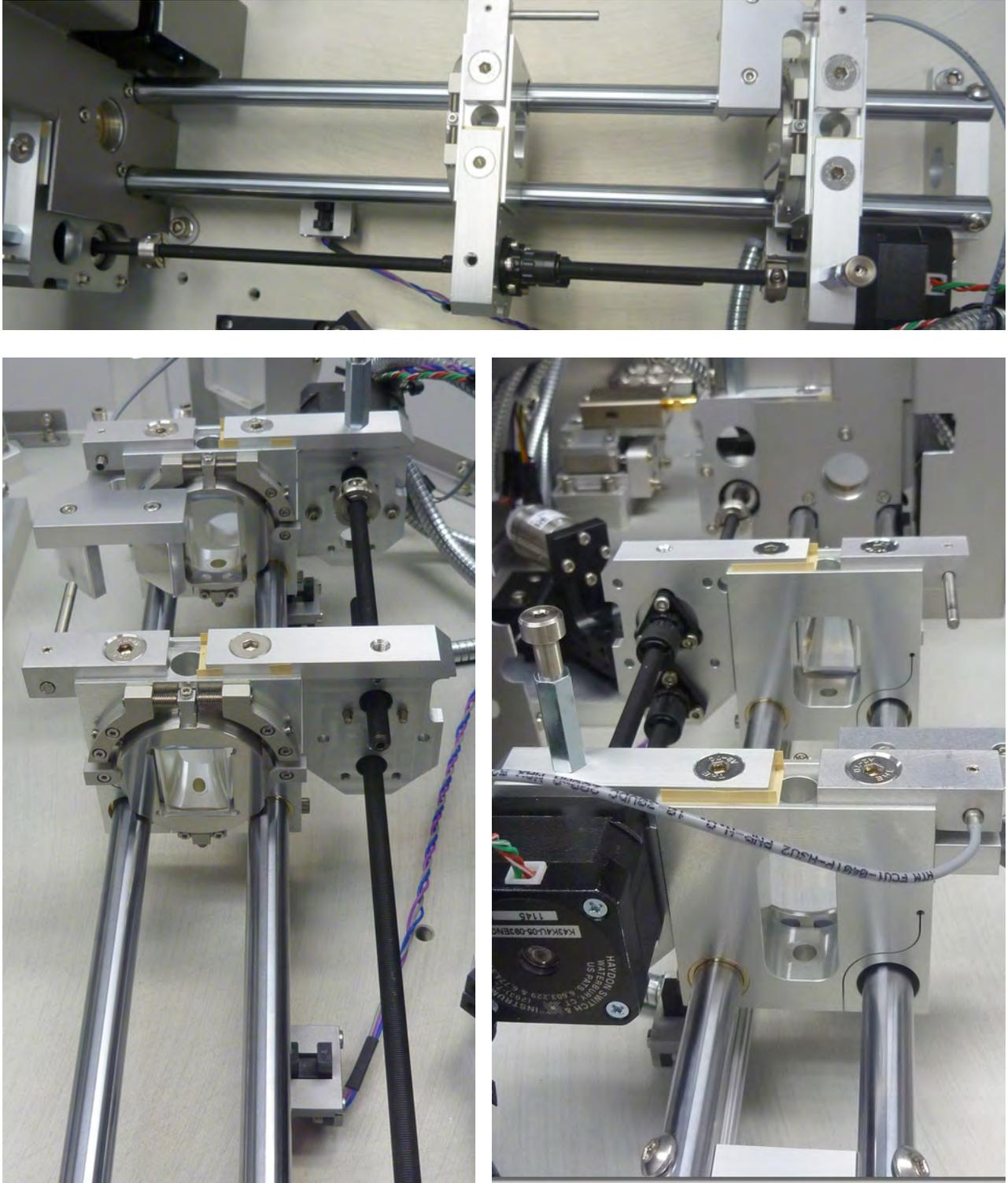
Figure 13. Top, front, and rear views of E4 and E5 carriers. Rails, motors, lead screws, limit switches, proximity switches, and E3 all visible.
